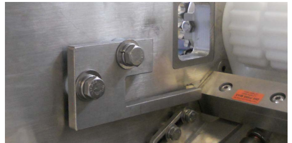
Stainless-steel rail catch safeguards against dropped pinblock to streamline maintenance.
