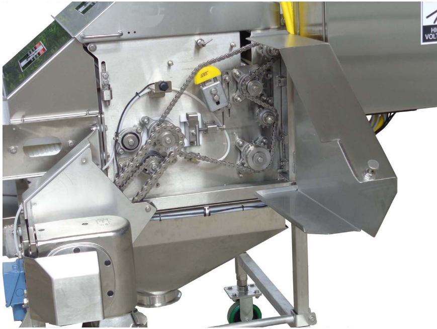
Allows easier access for drive system maintenance
