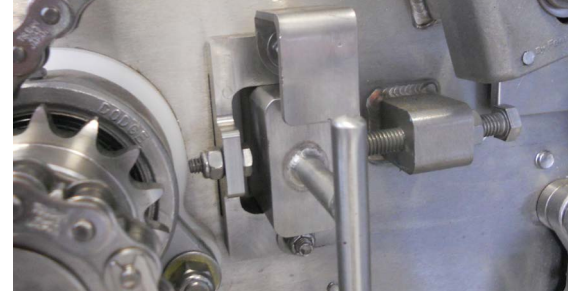
Positive-stop prevents overtightening the pinblock
